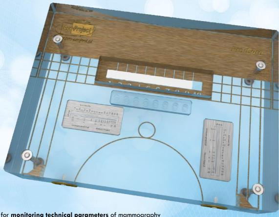
Pro-Euro phantom is used for **monitoring technical parameters** of mammography imaging systems according to the requirements of the **"European Guidelines for Quality Assurance in Mammography Screening"** and IEC 61223-3-2:
