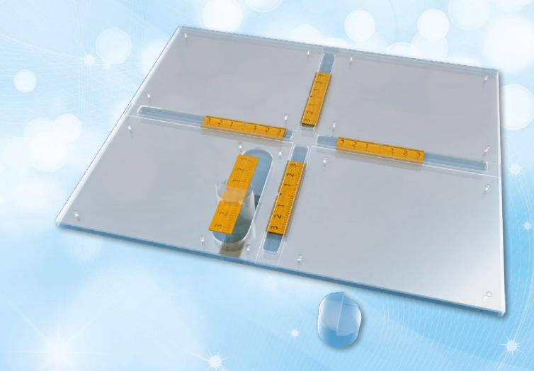
This test device was developed to provide the user with a convenient, quick and accurate way of testing collimation of mammography units. It is very simple to use. Instead of using all those hard-to-find coins, you only use our test tool.
