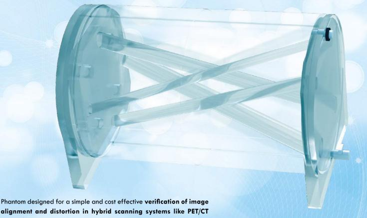
Phantom designed for a simple and cost effective verification of image alignment and distortion in hybrid scanning systems like PET/CT or NM/CT. It consists of a cylinder that can be filled with a variety of fluids. Several non-parallel rods of varying diameter and at certain angles in relation to phantom axes, run the entire length of the cylinder. Images produced with different modalities allow for quick and simple identification of misalignments on fused studies.
