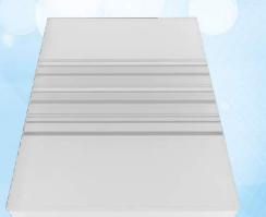
· Low Contrast Artery Insert containing 3 sets of analogue blood vessels (diameters 0.5, 1.0, 2,0 and 4.0 mm), each vessels group includes different iodine concentrations: 2.5, 5.0 and 10.0 mg/cc. Size: 203.2 x 152.4 x 25.4 mm
