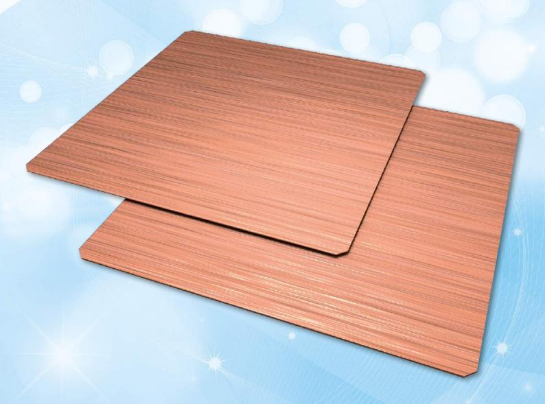
Set of high purity copper plates for testing Automated Exposure Control of radiography equipment. It can be mounted near the X-Ray tube and can be used instead of PMMA plates.
