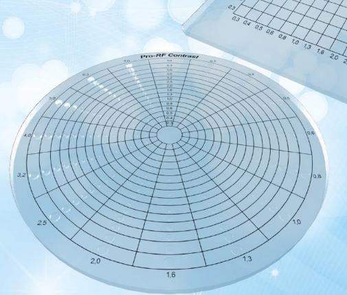
A Contrast-Detail (CD) phantom makes it possible to quantify both detail and contrast as observed by the radiologist. It can be used within the entire range of radiography diagnostic imaging systems, such as fluoroscopy and angiography. It has 225 holes that generate subtle changes in contrast.
