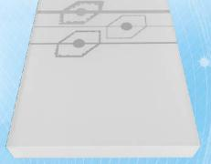
• 150 mg/ml lodine Artery Insert, 3 sets of analogue blood arteries (thickness 1.0, 2.0, 4.0 mm) each includes arteriarctial and arterial aneurysm which sizes are 1/4, 1/2 and 3/4 of artery diameter. Size: 203.2 x 152.4 x 25.4 mm
