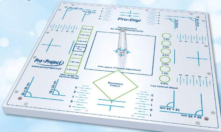
The Pro-Digi phantom is dedicated for acceptance and constancy tests of digital radiography equipment. It can be used to measure:
