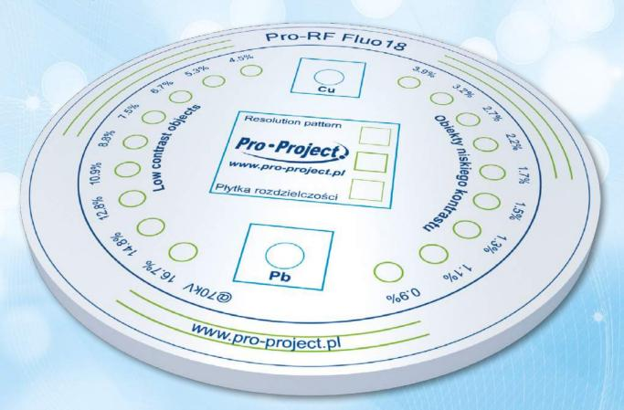
Phantom for evaluation of imaging performance of fluoroscopic systems. It allows for brightness and contrast adjustments, circular geometry check (scanning linearity) plus wide-range low-contrast and high-contrast resolution evaluation. Available in two standard layouts plus any custom configuration.
