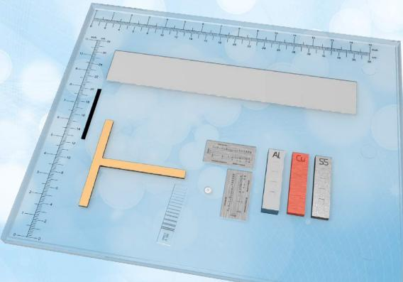
This Image Quality Indicator is used for testing all important parameters of CR scanner systems according to ASTM E 2445-05, ISO 16371-1 and EN 14784-1 standards. It provides means to measure: spatial resolution, unsharpness, contrast, MTF, laser beam jitter, scanner slipping and shading.
