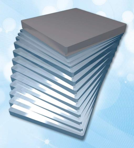
Set of acrylic plates for testing Automated Exposure Control of radiography equipment.
