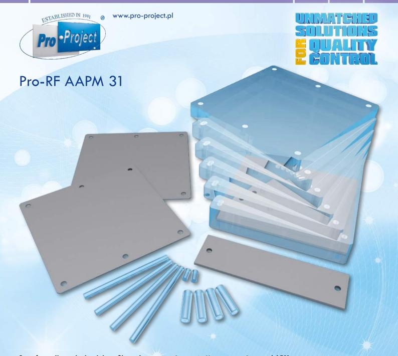
Set of acrylic and aluminium filters for testing diagnostic X-rays according to AAPM recommendations from Report No. 31 "Standardized Methods for Measuring Diagnostic X-Ray Exposure". Patient-equivalent acrylic and aluminium phantoms provide the necessary attenuation between the source and AEC or ABC detectors.
