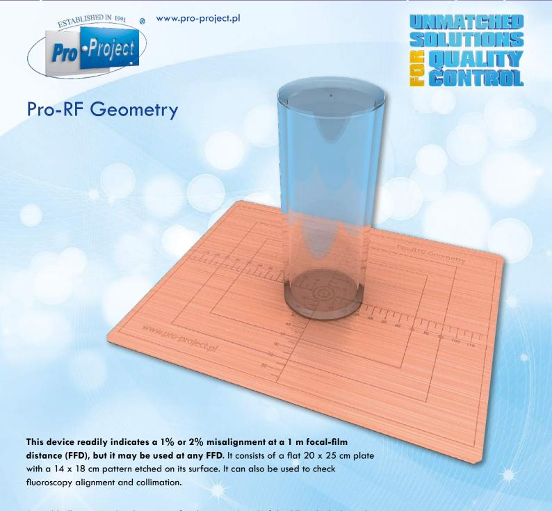
A steel ball is mounted in the center of a disc at each end of the 15 cm high clear plastic cylinder. When the balls are positioned over one another and at a right angle to the film, their images will appear as one if the central ray is truly perpendicular to the film.
