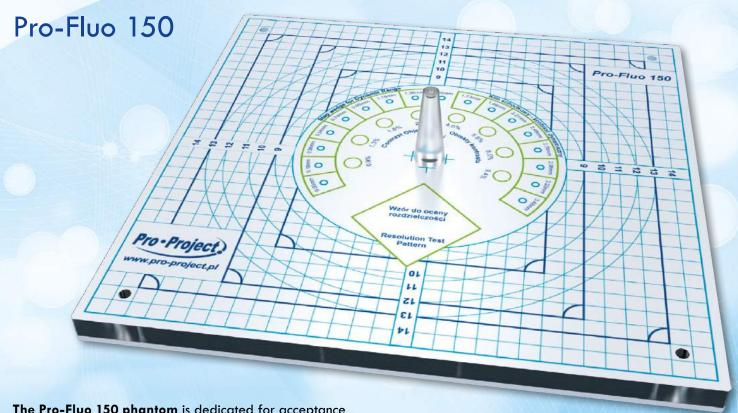
The Pro-Fluo 150 phantom is dedicated for acceptance and constancy tests of radiography and fluoroscopy equipment according to the new DIN 6868-150 standard.
