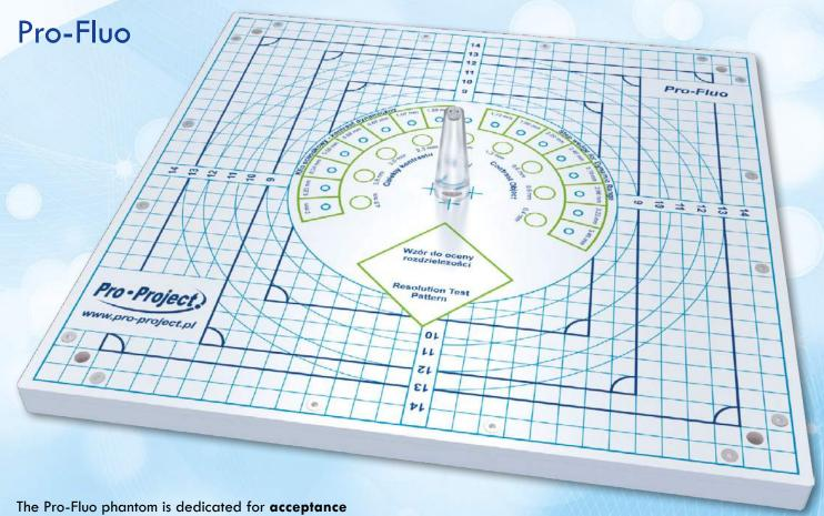
The Pro-Fluo phantom is dedicated for acceptance and constancy tests of digital and analogue radiography and fluoroscopy equipment. It can be used to measure:
