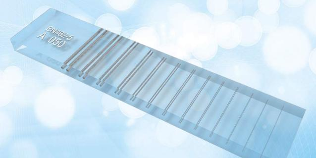
This Image Quality Indicator is especially made for digital X-ray applications. It may be used to evaluate image unsharpness (film and digital images) and basic spatial resolution in digital images according to EN 13068 (Radioscopy), EN 14784 and ISO 13671 (CR - Computed Radiography with imaging plates), ISO 17636-2 (digital radiography of welds - flat panel detectors) or ASTM E 2597 (characterization of digital detector arrays). It may also be used to determine focal spot sizes.
