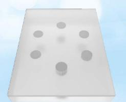
• Linearity Insert contains 6 iodine areas (19 mm diameter) having different iodine thickness and concentration: 0.5, 1.0, 2.0, 4.0, 10.0 and 20.0 mg/cm<sup>2</sup>. Size: 203.2 x 152.4 x 25.4 mm
