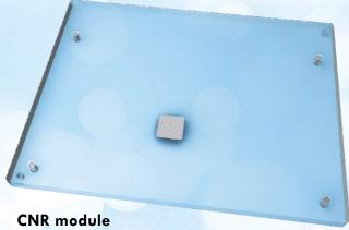
10 mm thick module containing a 20 x 20 x 0.2 mm aluminium filter, located 6 cm from the chest side
