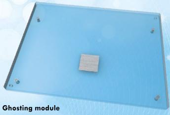
10 mm thick module containing a 30 x 30 x 0.1 mm aluminium filter for a ghost test
