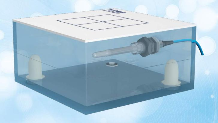
**Stationary water phantom** for high energy photon dosimetry with all types of ionization chambers.
