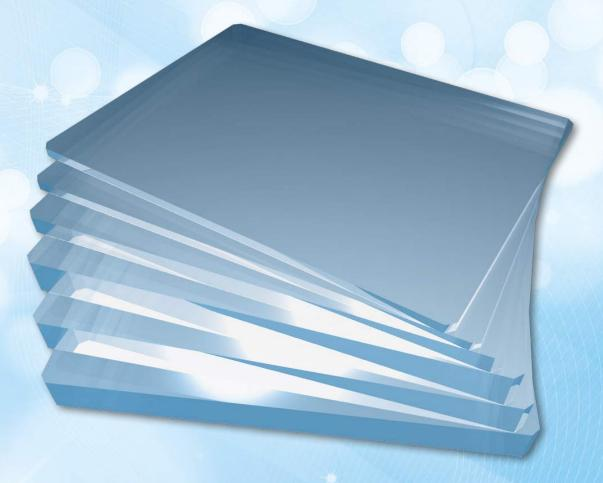
Set of acrylic plates for testing Automated Exposure Control of mammography systems.
