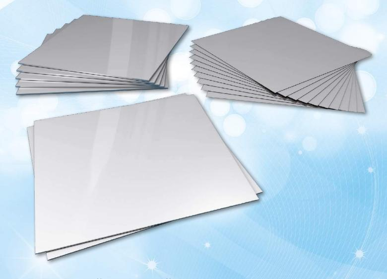
Different sets of high (99.9%) and standard (99.5%) purity aluminium plates for testing Half Value Layer.
